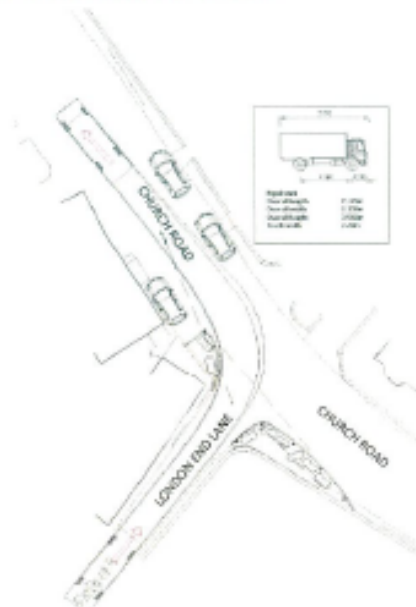
VEHICLE TRACKING AWAY FROM SITE 7.17m RIGID CHURCH LANE / LONDON END ROAD JUNCTION
